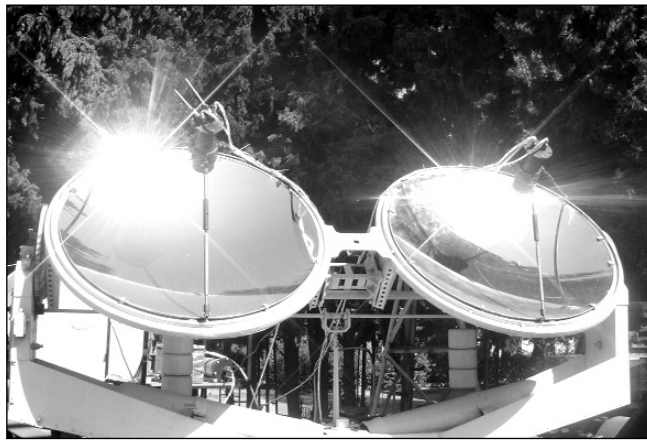
Figure 2. Solar plant with parabolic concentrator.
