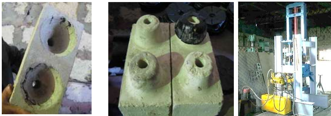
Fig. 4. Left, seismic resistant construction block (view from below); Center, seismic resistant construction blocks with damping pad applied; Right, machine for block production
