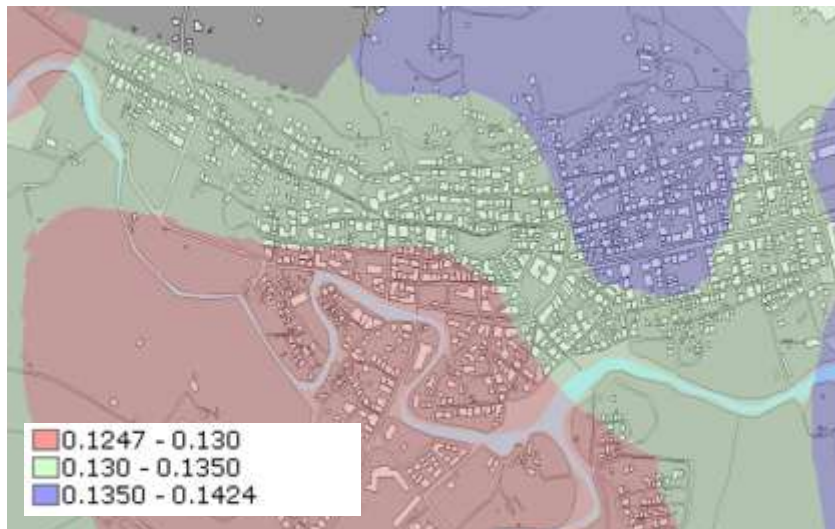
Fig. 3. Peak ground acceleration (PGA) map computed by a scenario earthquake in Grevena [19]
