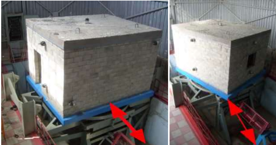
Fig. 8. Model building moving perpendicularly (left) and at a 30 degree angle (right), simulating two different seismic waves
