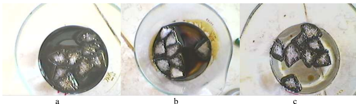
Fig.2. Photos of sorption of oil by integral sorbents on the basis of PE (a thickness of an oil film makes up 1 mm): a) the initial moment; b) in 15 minutes; c) in 60 minutes
