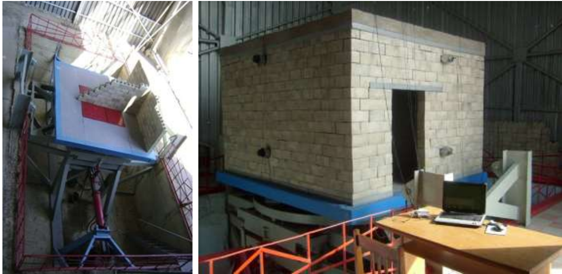
Fig. 6. Simulative seismic platform with test walls (left) and model building (right) on it
