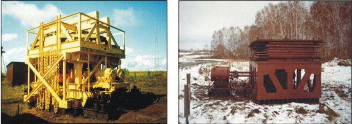
Fig. 2. 100-ton stationary and 40-ton mobile vibrator source
