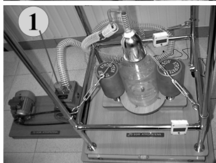
Photo 3-4. Vacuum pumps. 1 vacuum pump for creation of primary vacuum; 2 vacuum pump for creation of deep vacuum.
